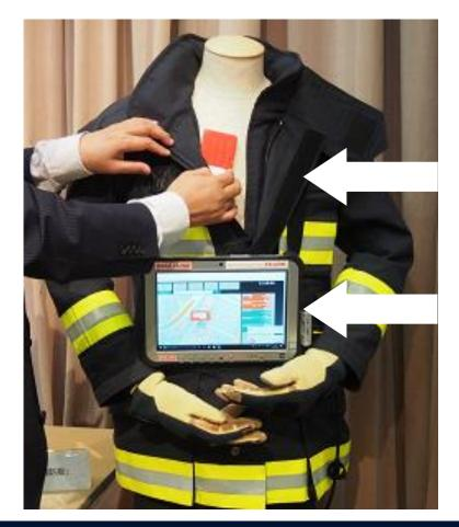
Attach a sensing device (red) to the inside pocket of the smart firefighter clothing.
